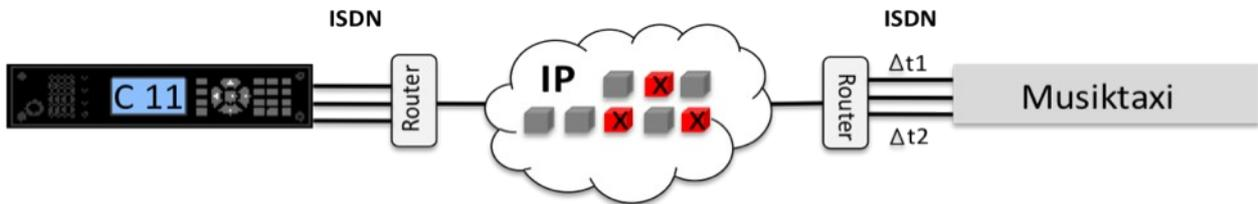
Figure 5 C11 and Musiktaxi via "ISDN via IP" with Bonding
