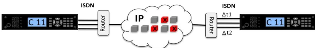
Figure 2 Two C11 Audio Codecs connected via ISDN, but ISDN is routed via IP incl. packet losses
